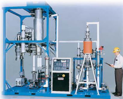
Turnkey, 12", stainless steel Wiped-Film Molecular Still Processing Plant with degassing stage, for edible oil deodorization
