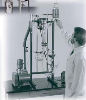
2", standard glass laboratory Molecular Still Unit for general R&D
