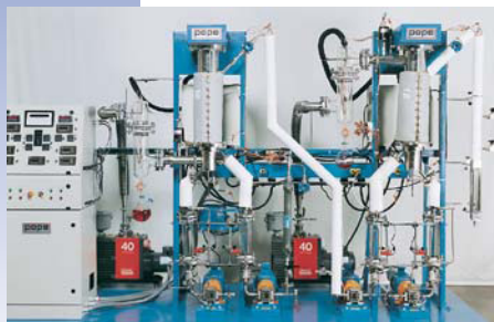
Turnkey, 6", two-stage Molecular Still Pilot Plant for long chain ester purification
