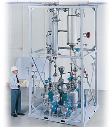
Turnkey, 12", stainless steel Wiped-Film Evaporator for polymer devolatilization
