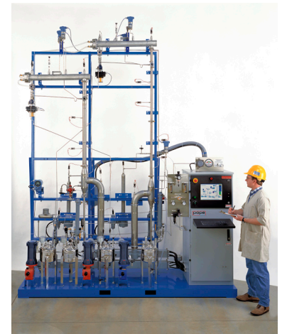
Complete turnkey 2-stage pressurizable Continuous Fractional Distillation System with 1 1/2" and 2 1/2" columns, thermosiphon reboilers, transfer pumps and receivers, explosion-proof PC-based control system.
