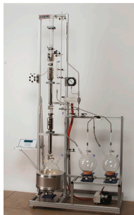
Batch vacuum distillation Column System with 2", 22 liter Autocol on a metal frame and additional vacuum assembly of 2 -12-L receiver flasks, pump system and gauges
