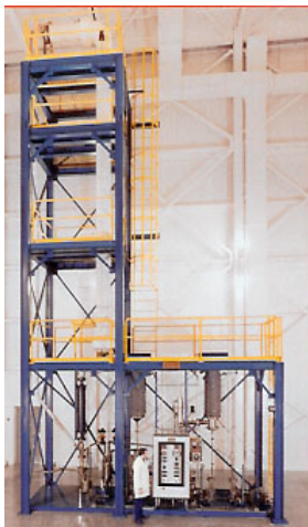
Pope Hybrid Distillation System, incorporating 12" diameter fractionating column with 10-square foot wiped-film evaporator for purification of heat-sensitive compounds. System also incorporates Molecular Still and explosion-proof control system.
