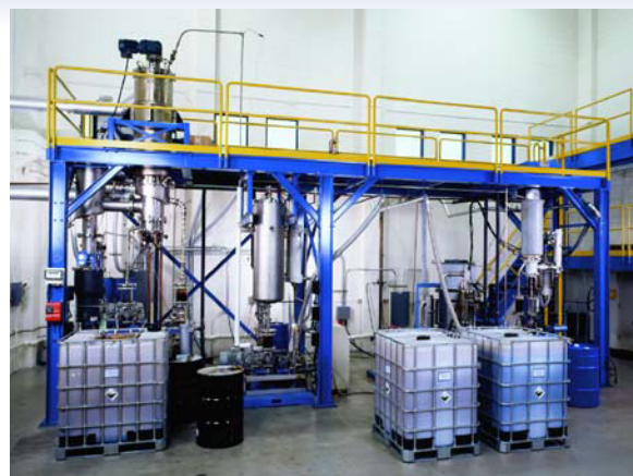
A Section of Pope's Wiped Film Still Toll Processing Area
